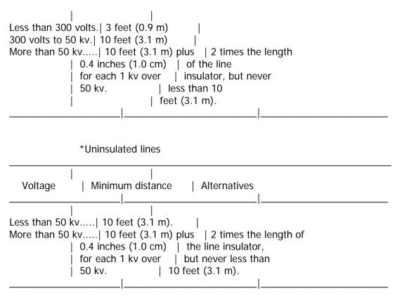
Exception to paragraph (f)(6): Scaffolds and materials may be closer to power lines than specified above where such clearance is necessary for performance of work, and only after the utility company, or electrical system operator, has been notified of the need to work closer and the utility company, or electrical system operator, has deenergized the lines, relocated the lines, or installed protective coverings to prevent accidental contact with the lines.
